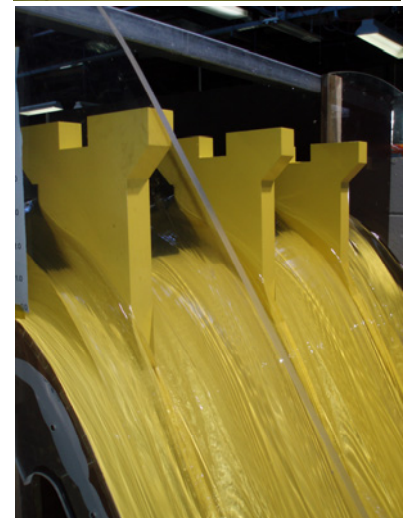
Water surface profiles on proposed piers
