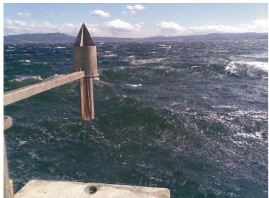
Radar water level monitoring sensor
