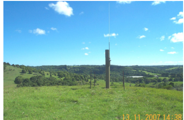
Installed rain gauge and radio data link
