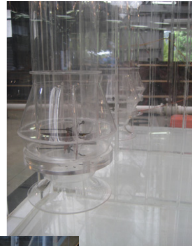
Bellmouth pump intake pipes
