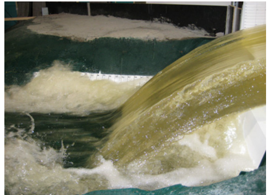
Flow exiting flip bucket into plunge pool area
