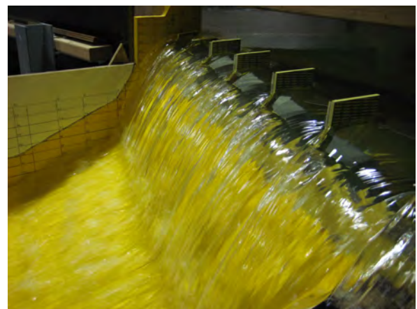
Lake Manchester spillway Hydroplus fusegate testing
