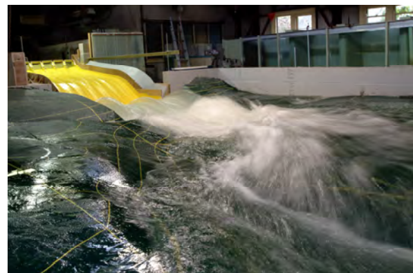
Burrendong Dam spillway physical model
